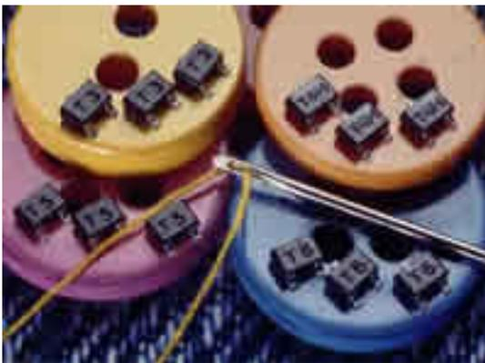
SMD devices are, by their very nature, too small to carry conventional semiconductor type numbers. Instead, a somewhat arbitrary coding system has grown up, where the device package carries a simple two- or three-character ID code.
